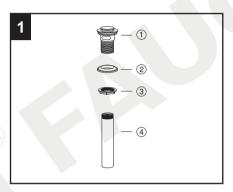
Unscrew grid drain body ① and tailpiece ④ . Romove rubber gasket ② from grid drain body ① .
