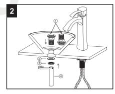
Apply plumber's putty to the underside of grid drain body ①, insert grid drain body ① to drain hole. Under basin, put back rubber gasket ②, tighten lock nut ③ with wrench tool. **Do not overtighten.** Clean excess putty. Wrap right mount of teflon tape to threads at the top of tailpiece ④, thread to the bottom of grid drain body ①. Hand tighten.
