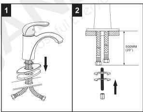
Connect blue marking hose ① to cold water supply, and red marking hose ② to hot water supply. Use wrenches to tighten connections.
