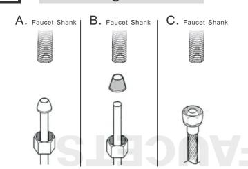
Connect to water supply lines with either:
